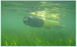
During the project, the use of **new ocean observing platforms** such as Autonomous Underwater Vehicles (AUVs) and Unmanned Aerial Vehicles (UAVs) will improve our capabilities to more accurately characterize complex environments and phytoplankton distribution from large scale patterns to small scale structures.
